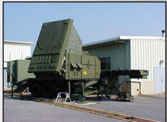
Letterkenny completes its first overhaul of a PATRIOT system, and is the only DoD installation overhauling and maintaining PATRIOT ground support equipment. The system contains seven different support pieces; PATRIOT Trailer Mounted Launching Station (LS), Radar Set (RS), Antenna Mast Group (AMG), Communications Relay Group (CRG), Guided Missile Transport (GMT), Information Coordination Center (ICC) and the Engagement Control Station (ECS).
